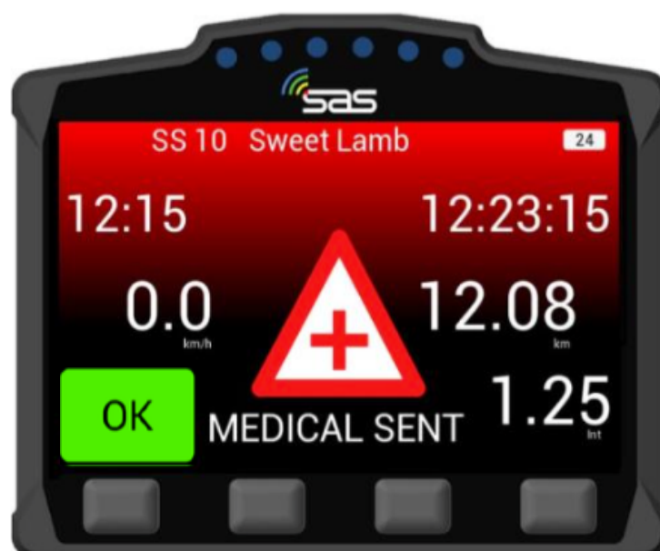
SCREEN 18: SOS confirmed, MEDICAL Assist required
